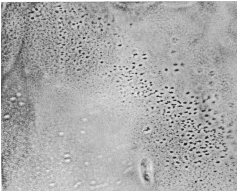
Figure 7. Acrylamide crystal given a radiation dose of 1.0 Mrad in a \text{Co}^{60} source at 500 000 rads/hr. Photographed 4 hr after irradiation. Phase contrast. Magnification, 960\times . The polymer nuclei lie in the 100 plane which is tilted with respect to the axis of the microscope. 4
